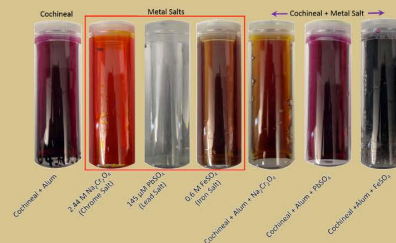
Figure 2: Picture illustrating the effect of mixing metal salts (i.e., chrome (Cr), lead (Pb), and iron (Fe)) with a cochineal and Alum solution. Adding 100 \mu\text{L} of 2.4 M chrome solution to the cochineal mixture produces a reddish-orange hue, 100 \mu\text{L} of 0.6 M iron solution results in a deep purple/black hue, and 300 \mu\text{L} of 145 \mu\text{M} lead solution yields a negligible color shift.
