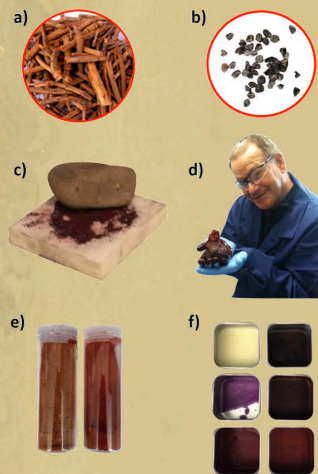
Figure 1: Raw (a) madder root and (b) cochineal. The raw materials were prepared by (c) grinding the matter into a powder and (d) steeping within a water bath for multiple days to release the pigment. While in solution, mordants, metal salts, and alkali salts were added to induce a color change. The solvent was then evaporated off and (e) the resulting product was crushed into a fine powder. (f) The powder was then set into a wax binder, which would be used for both a replicated painting of the Bearded Man and for optical analysis.
